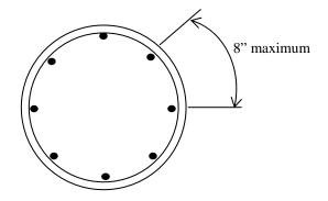
Interlocking spirals shall be used for non-circular columns. Reinforcement details are shown in the following sketch.
